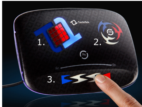
Device cover, front and back side: 1. LED-illuminated symbol window with animated effects, 2. Printed capacitive touch wheel, 3. Printed capacitive slider, 4. Printed circuitry. Source: TactoTek
